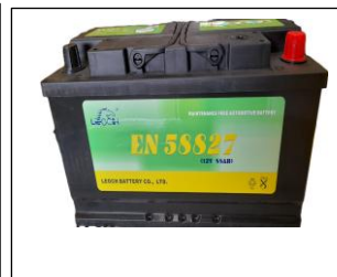
MF 58827 DIN88- BAT7015 (12V 88AH 154 Mins.) L=35 cms W=17.5 cms H=19 cms
